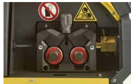
Professional double groove feeding mechanism with 4 rolls
