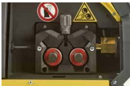
Professional double groove feeding mechanism with 4 rolls
