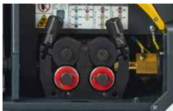
Professional double groove feeding mechanism with 4 rolls
